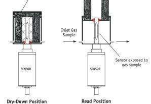
To allow rapid spot checks it is essential that the measuring sensor is kept drier than the sample to be measured.
