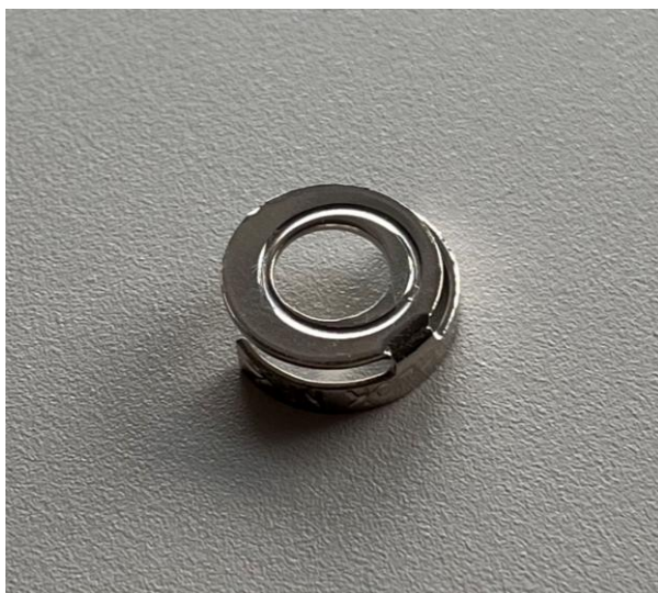
Misaligned Side Load VCR gasket
